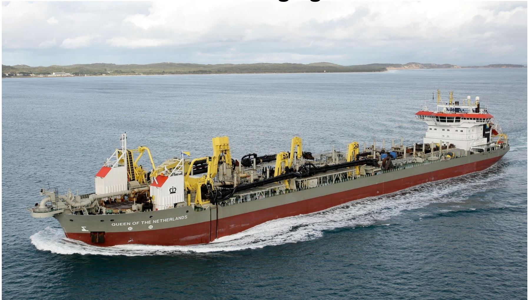
235m Conventional Trailing Suction Hopper Dredge
